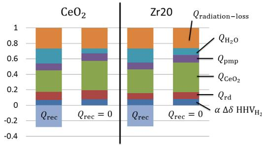
**Fig. 12** The relative heat consumptions calculated using the formulae  $\frac{Q}{Q_{\text{total}} + Q_{\text{rec}} + Q_{\text{radiation-loss}}}$  for both  $\text{CeO}_2$  and  $\text{Zr}_2\text{O}$ , at the optimal efficiency conditions seen in both figure 10 ( $Q_{\text{rec}} = 0$ ) and figure 11.
