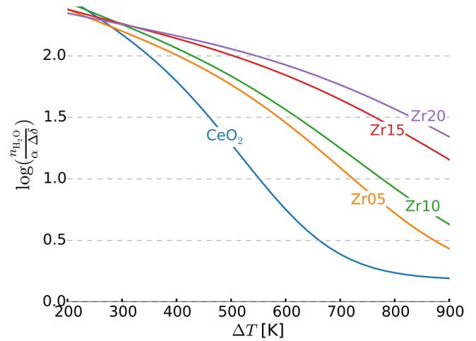
**Fig. 7** The number of moles of steam which are required per mole of hydrogen produced  $\log(\frac{n_{\text{H}_2\text{O}}}{\alpha \Delta \delta})$  vs.  $\Delta T$ . Here  $T_{\text{rd}} = 1773 \text{ K}$ ,  $p_{\text{O}_2} = 5 \times 10^{-4} \text{ bar}$  and  $\alpha = 0.96$  for  $\text{CeO}_2$  and  $0.92$  for the Zr added samples (see figure 9). The values of  $\delta_{\text{rd}}$  in order from  $\text{CeO}_2$ -Zr20 were  $0.03, 0.037, 0.041, 0.049$  and  $0.053$ .
