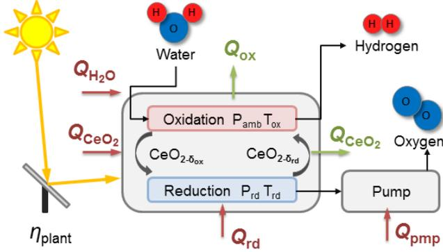
**Fig. 6** Schematic of the process showing the various heat inputs and outputs.
