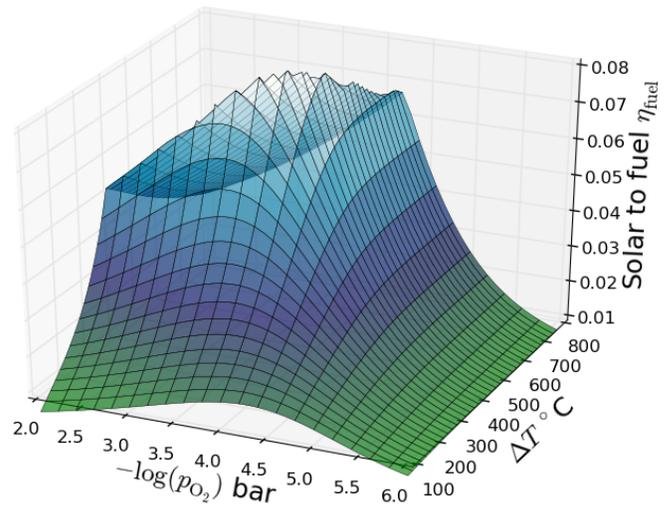
**Fig. 8** A plot of fuel production efficiency for pure  $\text{CeO}_2$  vs.  $\Delta T$  and  $p_{\text{O}_2}$ . Here  $T_{\text{rd}} = 1773 \text{ K}$  and the fraction complete  $\alpha = 0.96$ .
