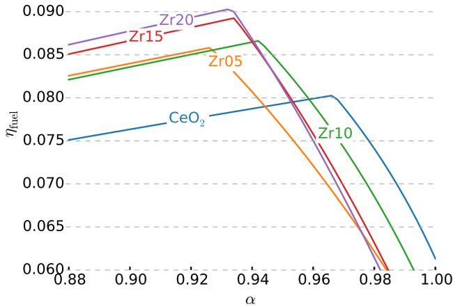
**Fig. 9** Solar to fuel efficiency for the different materials vs.  $\alpha$ , with heat recovery. The partial pressure at the end of reduction was set to  $p_{O_2} = 5 \times 10^{-4}$  bar,  $T_{rd} = 1773$  K and the optimal  $\Delta T$  values from figure 11 were used.
