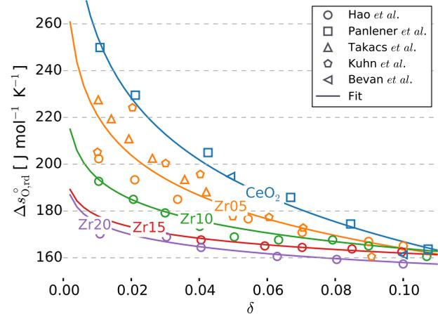
**Fig. 3**  $\Delta s_{\text{O,rd}}^{\circ}(\delta)$  fits for  $\text{CeO}_2$ <sup>7,37–39</sup>,  $\text{Ce}_{0.95}\text{Zr}_{0.05}\text{O}_2$ <sup>35,36,40</sup> and  $\text{Ce}_{1-x}\text{Zr}_x\text{O}_2$  for  $x=0.1, 0.15, 0.2$ <sup>35</sup>, are plotted along with some of the literature data.
