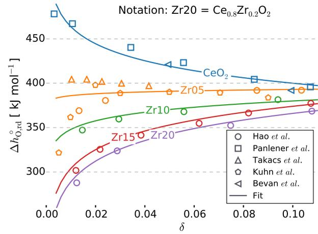
**Fig. 2**  $\Delta h_{\text{O,rd}}^{\circ}(\delta)$  fits of  $\text{CeO}_2$ <sup>7,37–39</sup>,  $\text{Ce}_{0.95}\text{Zr}_{0.05}\text{O}_2$ <sup>35,36,40</sup> and  $\text{Ce}_{1-x}\text{Zr}_x\text{O}_2$  for  $x=0.1, 0.15, 0.2$ <sup>35</sup>, are plotted along with some of the literature data.
