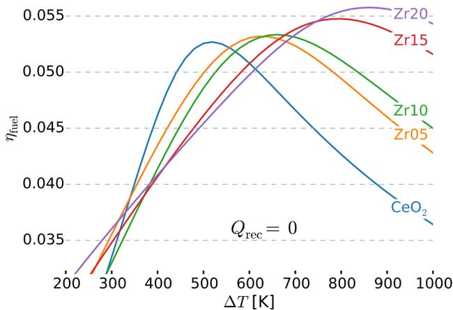
**Fig. 10** Solar to fuel efficiency for the different materials vs.  $\Delta T$ , without heat recovery. The partial pressure at the end of reduction was set to  $p_{O_2} = 5 \times 10^{-4}$  bar and  $\alpha = 0.96$  for  $CeO_2$  and 0.92 for the Zr added samples.
