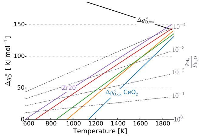
**Fig. 5**  $\Delta g_{O,ox}^\circ$  vs.  $T$  for  $\delta = 0.02$ . Also plotted are lines of  $RT \ln\left(\frac{p_{H_2}}{p_{H_2O}}\right)$ , with the pressure ratio indicated on the right axis.
