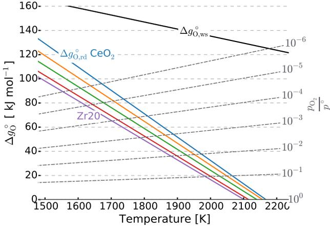
**Fig. 4**  $\Delta g_{O,rd}^\circ$  vs.  $T$  for  $\delta = 0.05$  (and for reference  $\Delta g_{O,ws}^\circ$ ). Also plotted are the lines of pumping work  $\frac{1}{2}RT \ln\left(\frac{p_{O_2}}{p^\circ}\right)$ , for a range of partial pressures labelled on the right axis.
