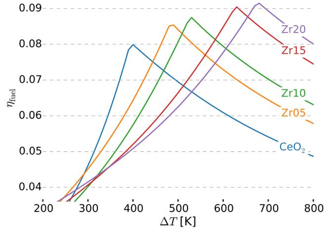
**Fig. 11** Solar to fuel efficiency for the different materials vs.  $\Delta T$ , with heat recovery from the ceria. The partial pressure at the end of reduction was set to  $p_{O_2} = 5 \times 10^{-4}$  bar and  $\alpha = 0.96$  for  $CeO_2$  and 0.92 for the Zr added samples.
