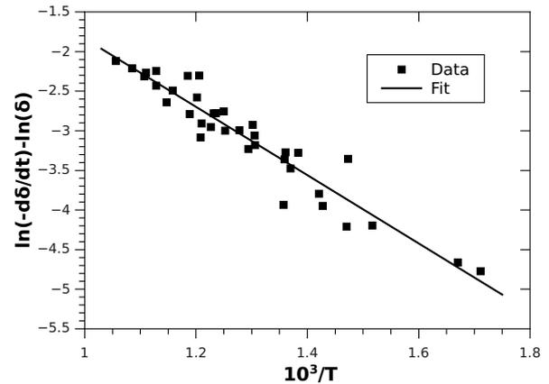
Figure 9: A plot of  $\ln(k)$  vs.  $\frac{10^3}{T}$ . These points are from several different scans with the final temperatures reached in the range 500 - 1000 °C.
