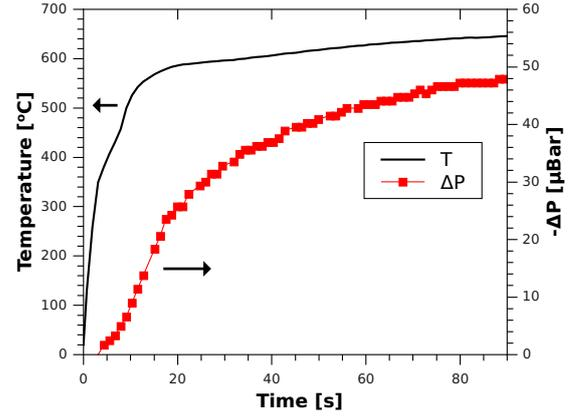
Figure 8: A graph showing sample temperature and the drop in pressure for the re-oxidation of a Ceria pellet.
