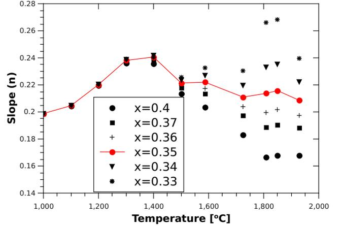
Figure 2: The slope obtained from a linear fit of  $\log\left(\frac{\delta}{x-\delta}\right)$  vs.  $-\log(P_{O_2})$  plotted against temperature for six different values of the parameter  $x$ .
