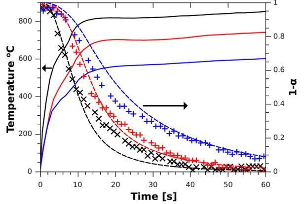
Figure 10: Experimental temperature and the corresponding fraction of remaining oxygen vacancies for three different input powers. The solid lines are the temperature, the crosses are the experimental fraction of remaining oxygen vacancies and the dashed lines are those predicted by equation 21.
