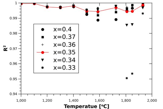
Figure 3: The  $R^2$  value obtained from a linear fit of  $\log\left(\frac{\delta}{x-\delta}\right)$  vs.  $-\log(P_{O_2})$  plotted against temperature for five different values of the parameter  $x$ .
