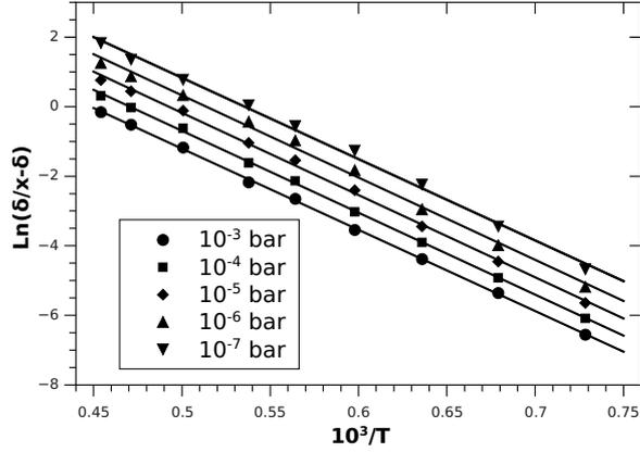
Figure 4: A graph of  $\ln\left(\frac{\delta}{x-\delta}\right)$  vs.  $\frac{10^3}{T}$  for a range of different pressures. The data is again taken from Panlener et al[29] and Zinkevich et al[24]. The data was fit linearly and from the slope of each line we can calculate the difference in activation energies  $\Delta E$
