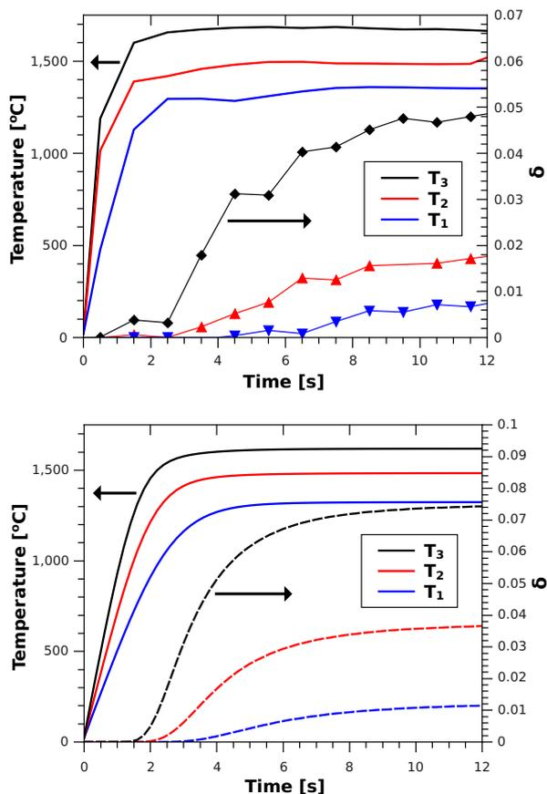
Figure 11: Top: Experimental temperature and the corresponding measured  $\delta$  for three different input powers. Bottom: A numerical model with similar temperature curves and the corresponding numerical rates predicted.
