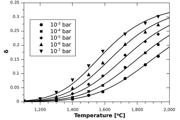
Figure 5: A plot of the vacancy concentration  $\delta$  vs. temperature. The points are the same as Figure 4, plotted with the results of fitting the analytical model to the same data.
