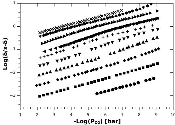
Figure 1: Isothermal plots of  $\log\left(\frac{\delta}{x-\delta}\right)$  vs.  $-\log(P_{O_2})$  with the value of  $x$  set to 0.35. The temperatures plotted are from bottom to top  $1000, 1100, 1200, 1300, 1400, 1500, 1587, 1725, 1850,$  and  $1930^\circ\text{C}$ . The data is taken from Panlener et al [29] and Zinkevich et al [24].
